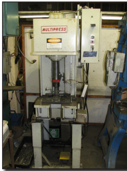
The point-of-operation on this hydraulic press is unguarded and poses a crushing/amputation hazard to the operator. (IOSHA photo)
