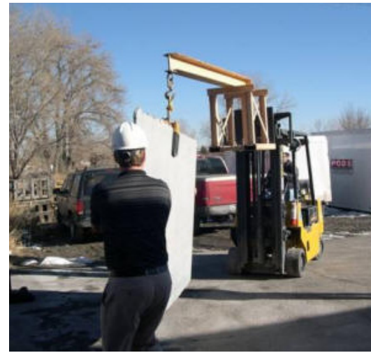
Safe slab transport: An employee stays out of the way of the stone slab's fall shadow during transport. (Photo taken from www.osha.gov )
