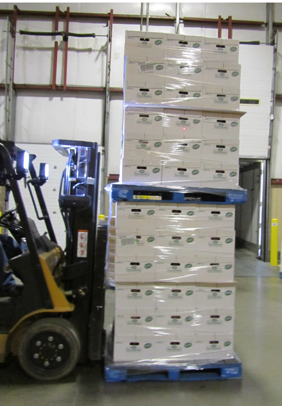
A forklift in operation is "dragging" the bottom pallet. Additionally, the load weighs more than the forklift's rated capacity. (Photo taken by IOSHA Compliance Safety and Health Officer Laura Groom)
