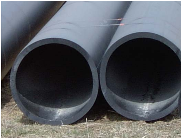
Figure 3 – “Thick-walled” small diameter HDPE pipe.
