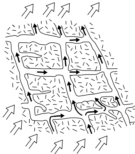
Figure 8. Ground-Water Flow and Dissolution Features of Carbonate Rocks.
