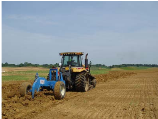
Using a ripper to break up compaction on reclaimed land. Photo courtesy of Peabody Coal
