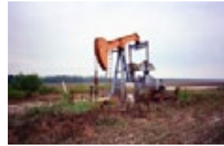
Crude oil pumping unit
