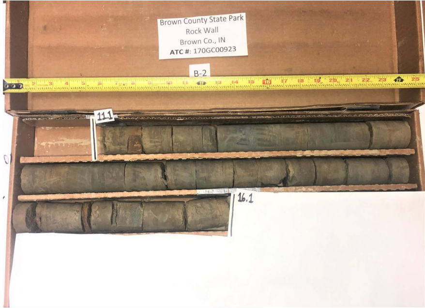
Figure B-2.1 Rock Core #1 11.1' to 16.1' Recovery = 92% Rock Quality Designation (RQD) = 32%
