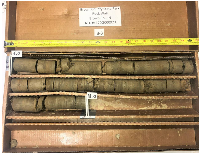
Figure B-3.1 Rock Core #1 6.0' to 11.0' Recovery = 96% Rock Quality Designation (RQD) = 29%
