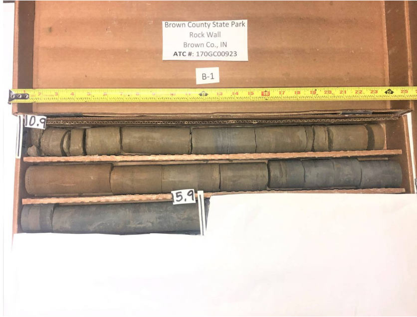
Figure B-1.1 Rock Core #1 10.9' to 15.9' Recovery = 98% Rock Quality Designation (RQD) = 44%
