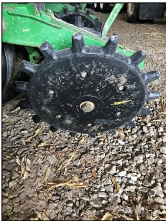
Figure 2. Closing wheel equipment modification for no-till corn and soybean planting.
