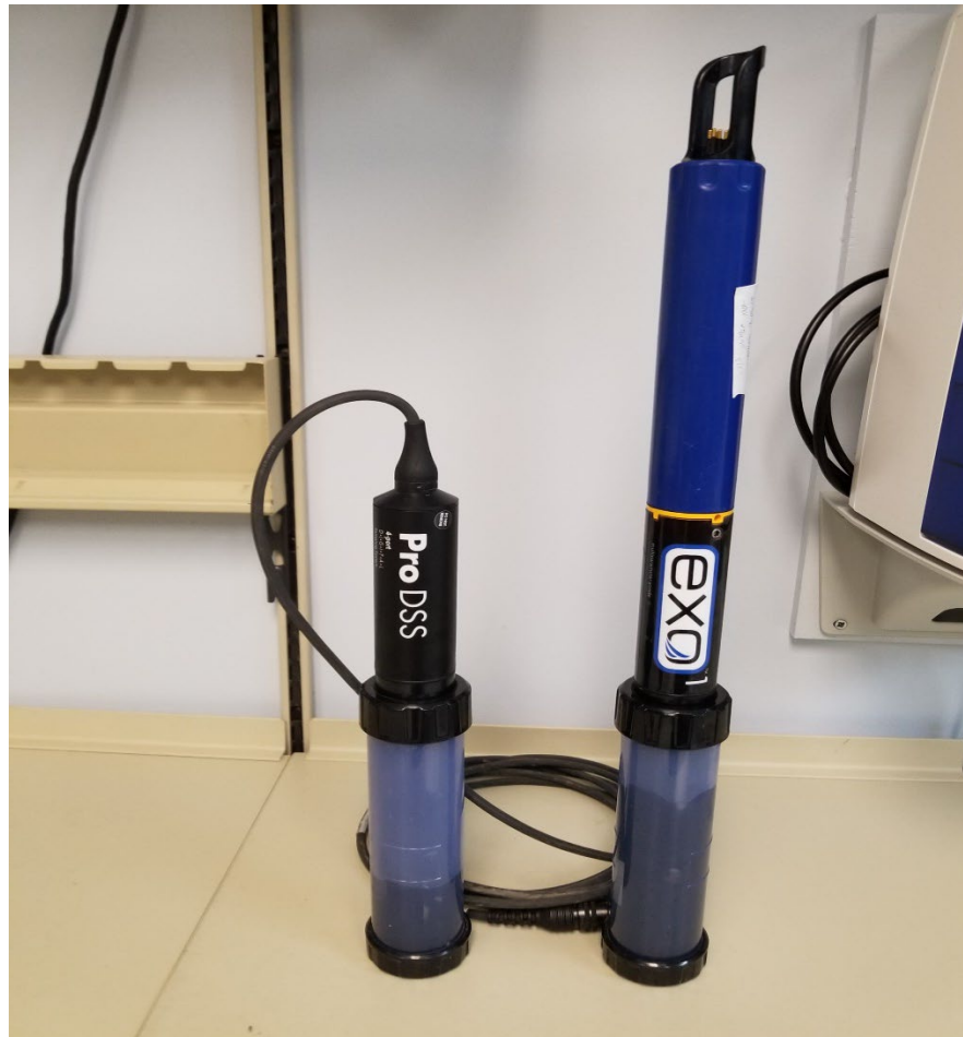
Figure 4. Image of a ProDSS sonde with Cable Assembly and Calibration Cup Attached and an EXO sonde with Calibration Cup Attached.
