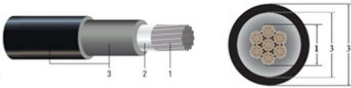
2kV HDFPC-DLO, RHH/RHW-2 & RW90
