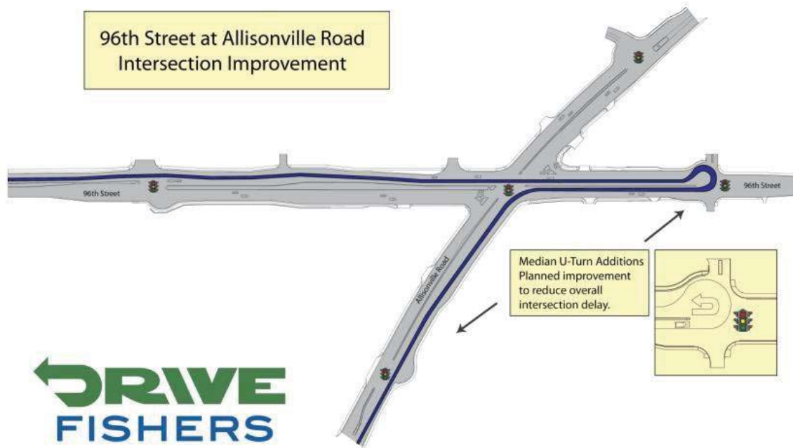
Figure 2- Example of Median U-turn
