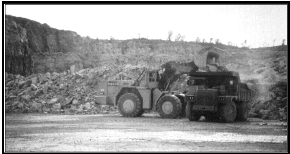
Figure 5-4. Loading Quarry Truck
