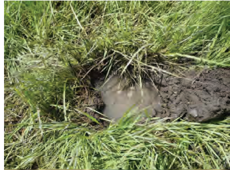
Picture 391: Upland area, DP91 – pit with water present just below the surface, 05/07/2020 (Exhibit 6V)
