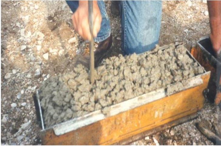
Figure 3-3 Concrete Beam Used for Flexural Testing
