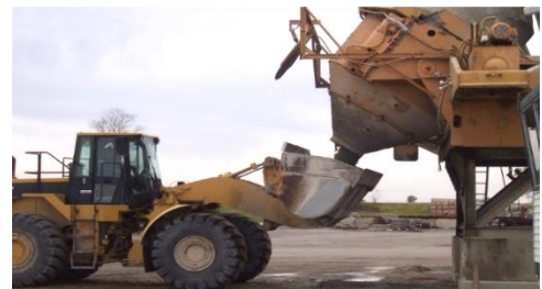
Figure 3-6 Loading a bucket
